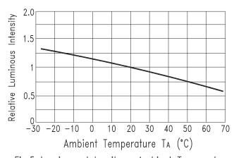
Fig.5 Luminous Intensity vs.Ambient Temperature
