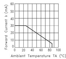
Fig.3 FORWARD CURRENT DERATING CURVE
