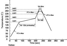
We recommend the soldering temperature 245± 5  $^\circ$ C; The maximum temperature should be limited to 260  $^\circ$ C.
